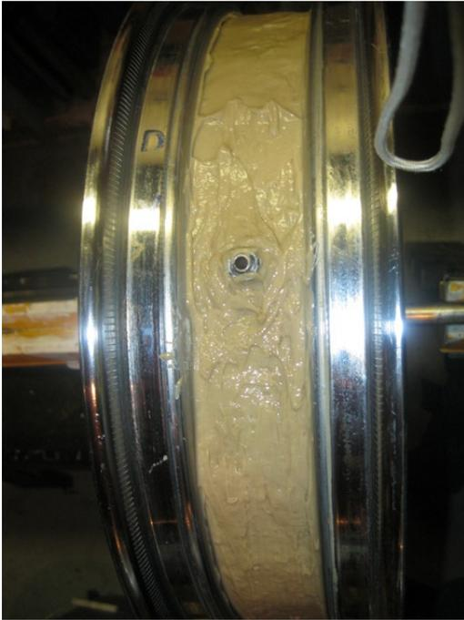
7. Allow the sealant to completely cure (5 to 7 days) in a high humidity environment. If the humidity level is low, place the rim in a plastic bag with a bucket of water or wet towel and close the bag.
