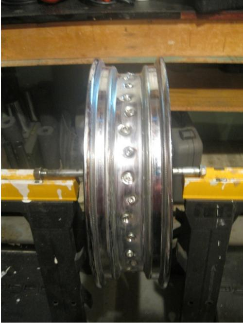
2. Using very coarse sandpaper, scuff up the center trough of the rim, especially the sides. This will ensure the sealant's proper adhesion to the rim.
