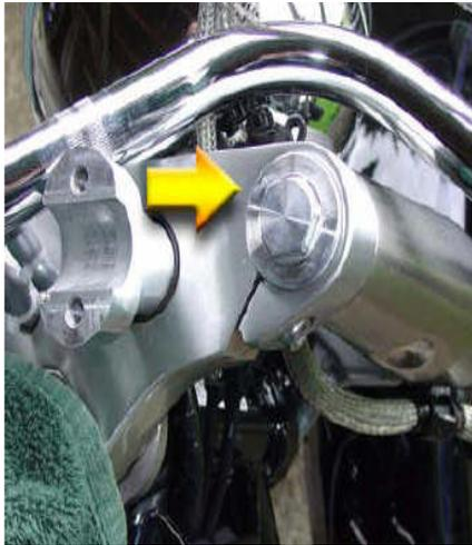
3. Pull out the metal factory spacer tubes. Use a wire hanger with a bend on the tip to fish out the springs. Pull then out slowly, they will come out dripping oil. Save the washers that rest on top of the springs - these serve as a base for the spacer tube.
