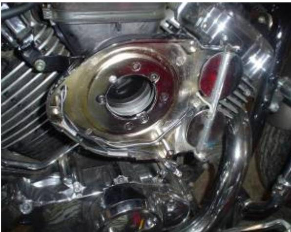
Start out cutting the rubber bushings off of the LEDs; you will not need them for this installation. Then, insert the LEDs in the rear drain hole of the Hypercharger and use the double stick tape to hold them in place. I put one of the LEDs in the front of the Hypercharger, just behind the butterflies.
