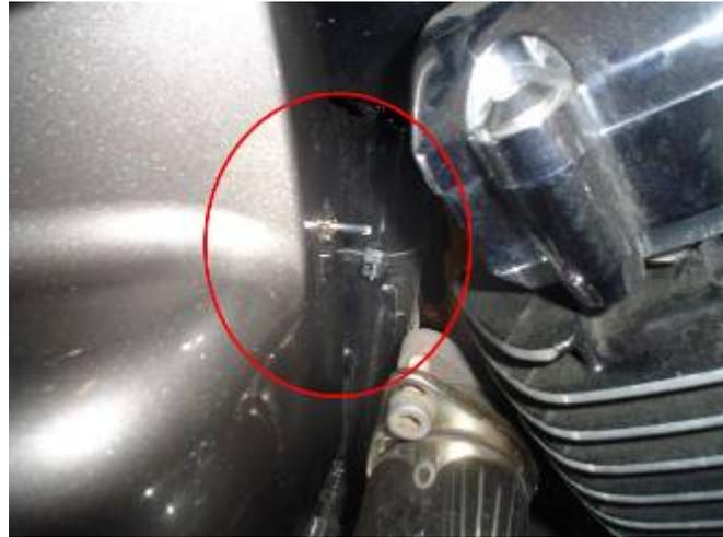
I drilled a small hole (*1/4"*, I think; *just measure up the top of the switch with a drill bit. You'll be able to tighten it down enough if the hole's a hair big*) in the battery cover and assembled the switch in the cover.
