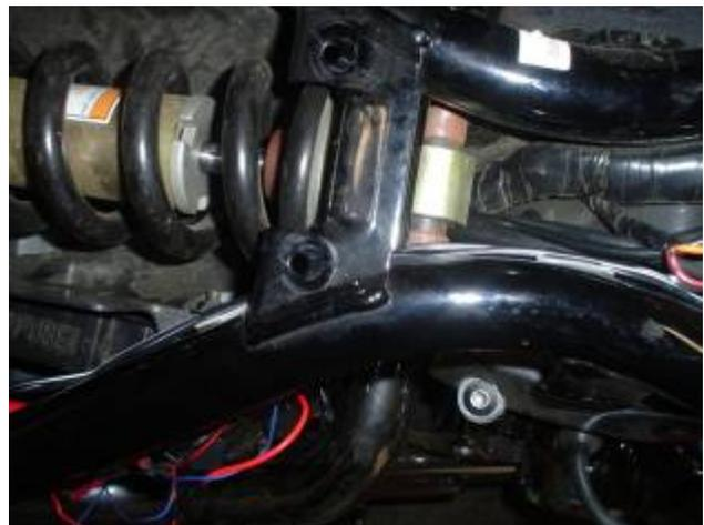
*(It might be easier for some to start at the rear of the bike and work forward towards the Hypercharger, which is fine; just remember not to leave too much wire at the front.)*
