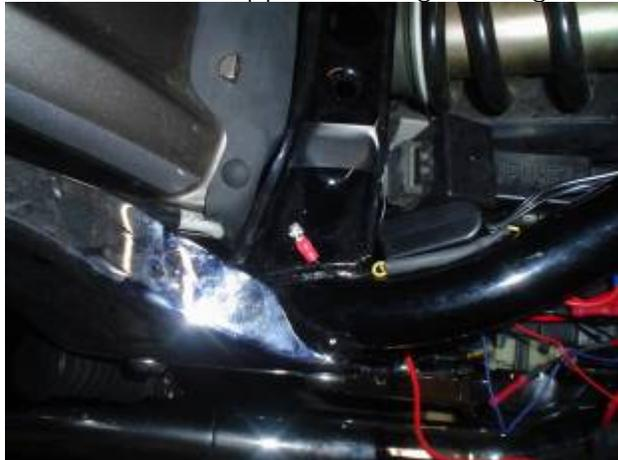
I had a screw already, so I just drilled a hole through the metal to match the size of the screw. I also crimped a ring terminal onto the end of the wire so that the wire would not come off the ground screw.
