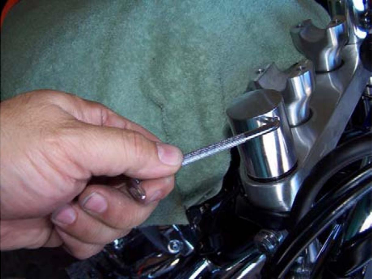
Once both sides are installed, you have to loosen the clamps on the triple tree and slide the forks down. On my Custom, there were five things I had to loosen per side. The top and bottom clamps, the Turn Signal bracket (two screws) and the two clamps for my Memphis Fats windshield. Here are shots of the top, bottom and Turn Signal clamps.
