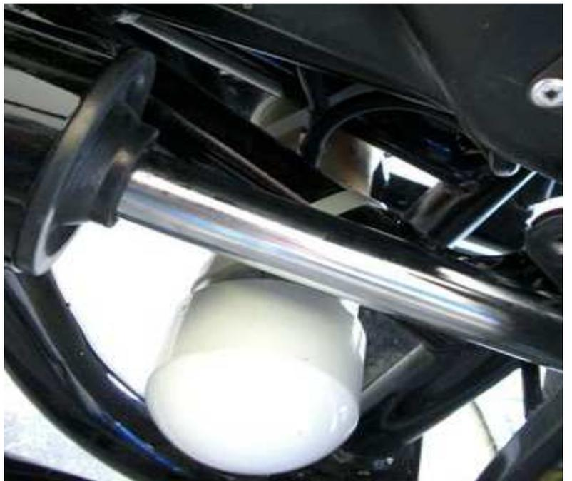
Drill two 5/16" holes in the pipe, tap(1/8") them and insert brass 3/16" nipples for your vacuum hose. (2568)
