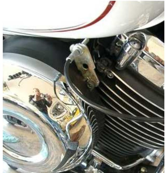
I used the long "cable" and no bead chain to connect to the throttle. (2560)
