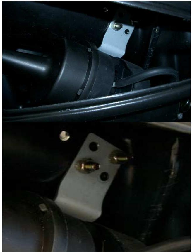
I made the hole in the front of the box (where the servo cable goes through) way too large, but I wasn't sure what angle it would be at when I installed it, so I kept cutting it bigger so the cable wouldn't be bent too sharp. (2565)
