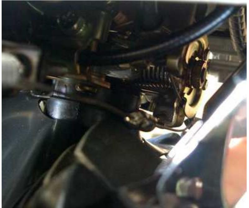
Spread the other end and hook it to the servo cable and then using your pliers, close it again.
